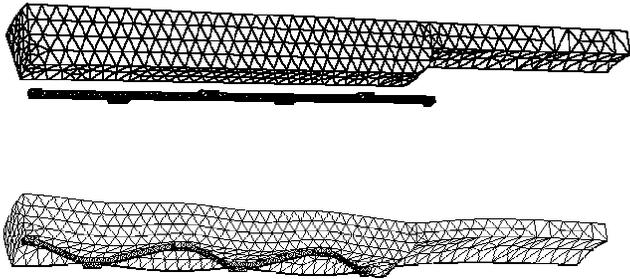
Figure 3. Undeformed (top) and deformed (bottom) mesh configurations of the stented artery after the expansion for model B.
