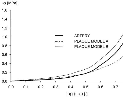
Figure 2. Stress-strain curves for the artery (bold) and the two models of plaque with increasing stiffness.
