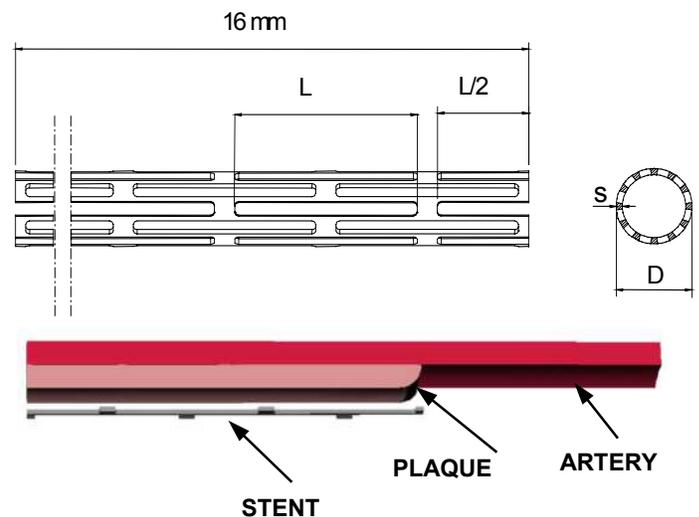
Figure 1. Geometry with the main dimension of the stent and a twelfth of the whole unexpanded model of the stent strut with the correspondent portion of stenotic coronary artery. L: length of the slot, s: thickness, D: outer diameter.
