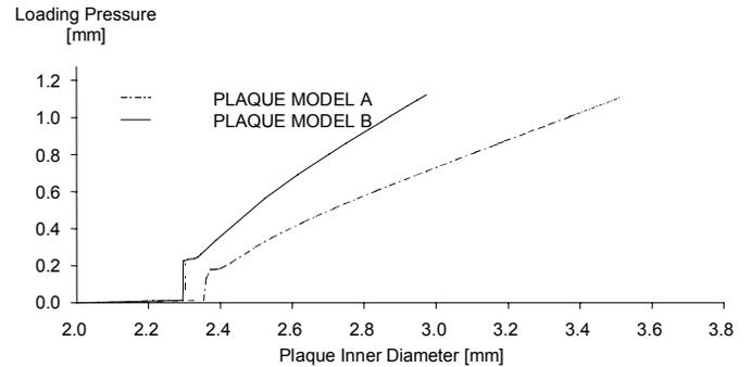
Figure 5. Pressure-inner expanded diameter curve for the two models adopted.
