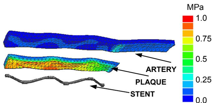
Figure 4. Von Mises stresses in the artery and in the plaque in an exploded representation of the model B. The stent is represented without reporting the Von Mises stress which are greater of two orders of magnitude (about 350-400 MPa).
